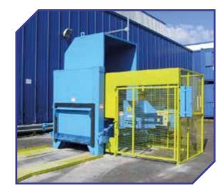
The KHD 5000 is a high performance compactor. A reliable and proven machine that can be used to compact large bulk waste on large industrial sites. This machine offers an even wider charge box making it ideal for larger waste throughputs. The 5000 comes as standard with high safety features including low 24v operating controls, dual safety monitoring circuits and E-stops at control positions.
